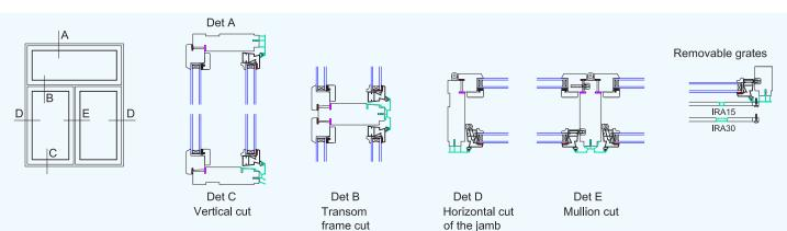
The WNE-A energy windows in the Watt series are of either energy class A or B, depending on the glass options chosen. The bevelled shape of the inner sash in these models makes Lammin's sturdy, energy-efficient inner sash appear more elegant, and the rectangular surface fitting selected for the model matches the style. The windows are manufactured per the requirements indicated for the customer and the construction site. They are suitable for new structures and repair/renovation projects alike.
