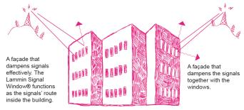
When the wall elements dampen the signals more effectively than the windows, the windows function as a route/opening through which the signals can get inside the building. In that case, regular energy-efficient windows may prevent signals from entering the building. When it comes to indoor reception, the big picture is what matters.
