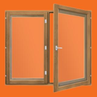
Eko Watti is the first A++ rated energy efficient window with an opening function on the market (as classified by Motiva). It has **quadruple glazing** and a **unique**, **protected outer frame structure** (PRH FI 7415/2007). Annual energy consumption is just 42 KW per square metre of window, with a U-value of 0.66.
